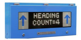
The PD8.2 is designed and approved to be used in hazardous (explosive) gas atmospheres that may be encountered in coal mines and petrochemical installations. It carries both ATEX and IECEx accreditation and is certified intrinsically safe to both Group I (Ex ia 1 Ma) and Group II (Ex ia IIB T4 Ga) and also tested to **IP65**.
